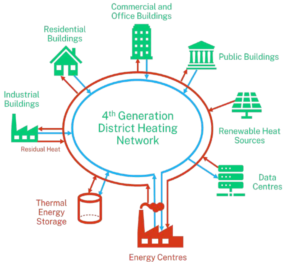
Figure 5: Conceptual 4th Generation District Heating Network
