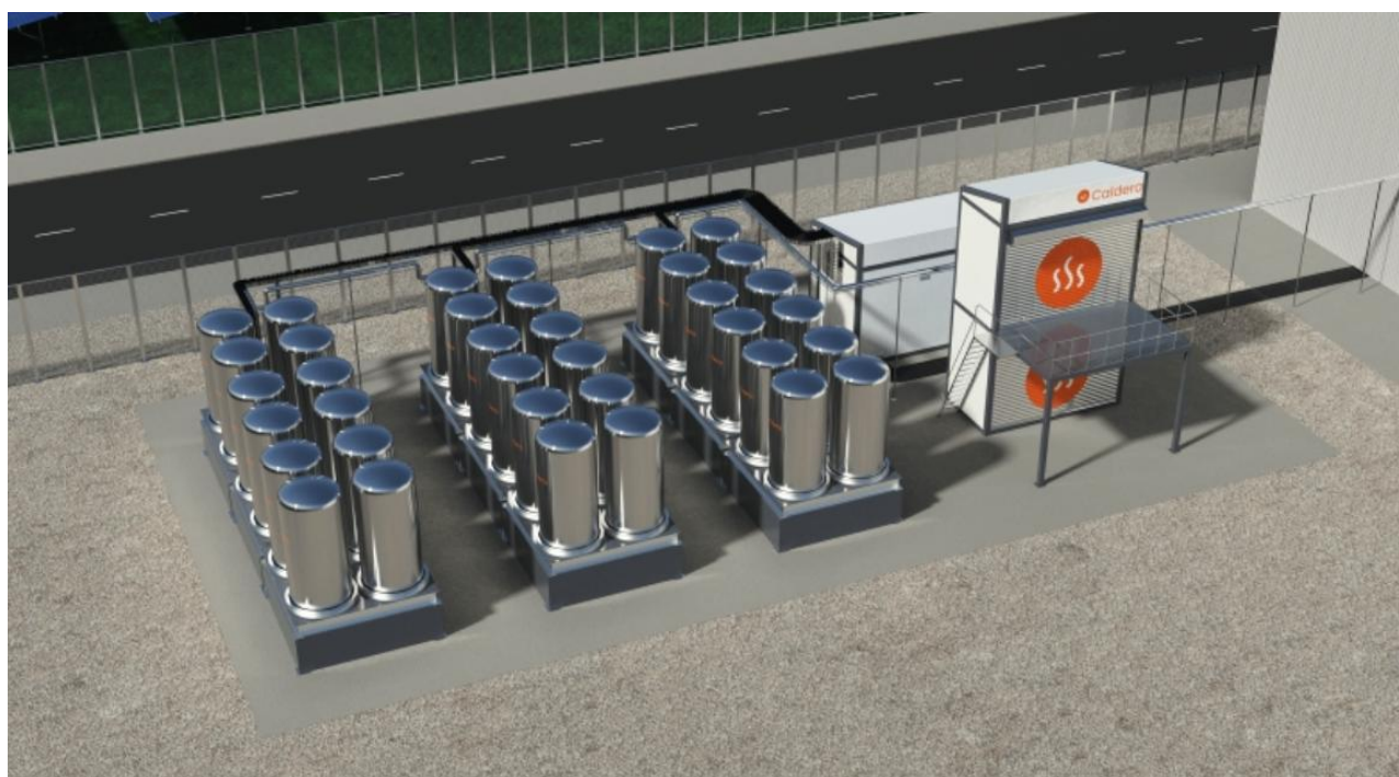
Figure 12: Caldera's system pilot demonstrator, industrial-scale heat cells made from volcanic rock and scrap aluminium 21
