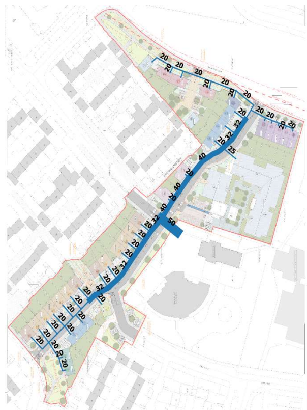
Figure 23: Map Showing DH Pipe Diameters - Low Density Residential Development Example
