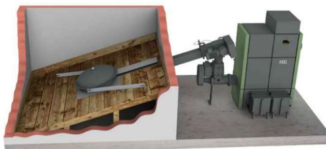
Figure 9: Wood Pellet Bulk Storage & Boiler – Courtesy of HDG & Glas.ie
