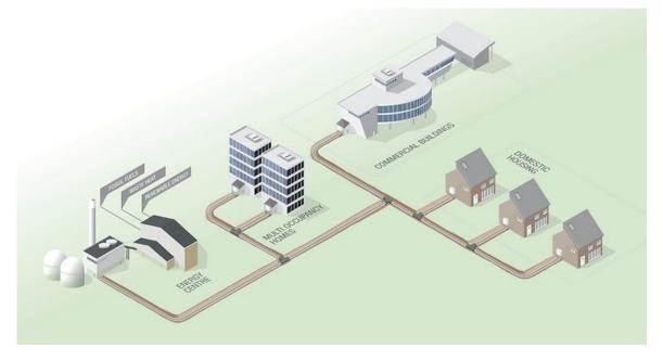
Figure 7: Indicative Diagram of a District Heating System (Source: REHAU)
