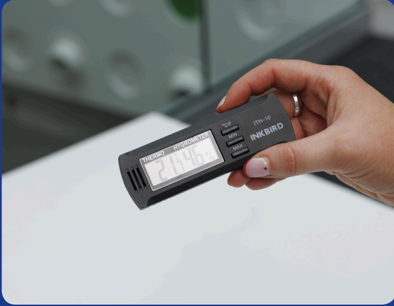
Temperature and humidity meter Checks room temperature and air humidity
