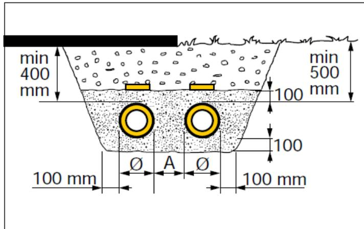
Figure 32: Indicative Trench Dimensions (source: Logstor Design Manual)
