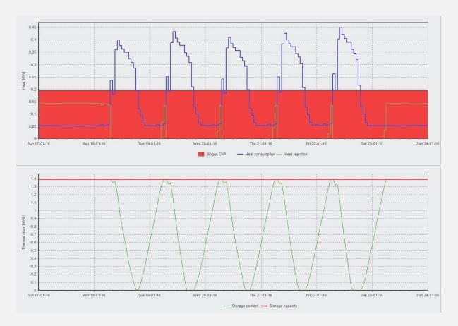
Figure 17: Production graphic; Biogas CHP, heat rejection and thermal store
