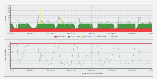
Figure 7: Production graphic; CHP, back-up boilers and thermal store
