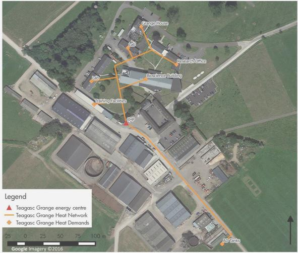
Figure 16: Teagasc Grange CHP and proposed DH network
