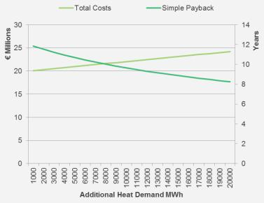
Figure 9: Effects of additional heat demand on the system costs and payback
