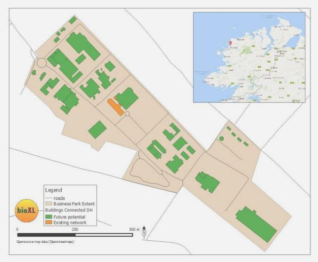
Figure 40: Existing and potential heat network customers
