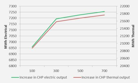
Figure 6: Optimising Size of Thermal Storage
